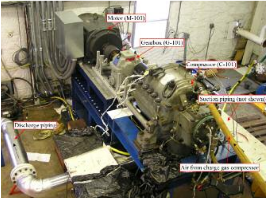
FIGURE 10.12. Centrifugal compressor test stand.
