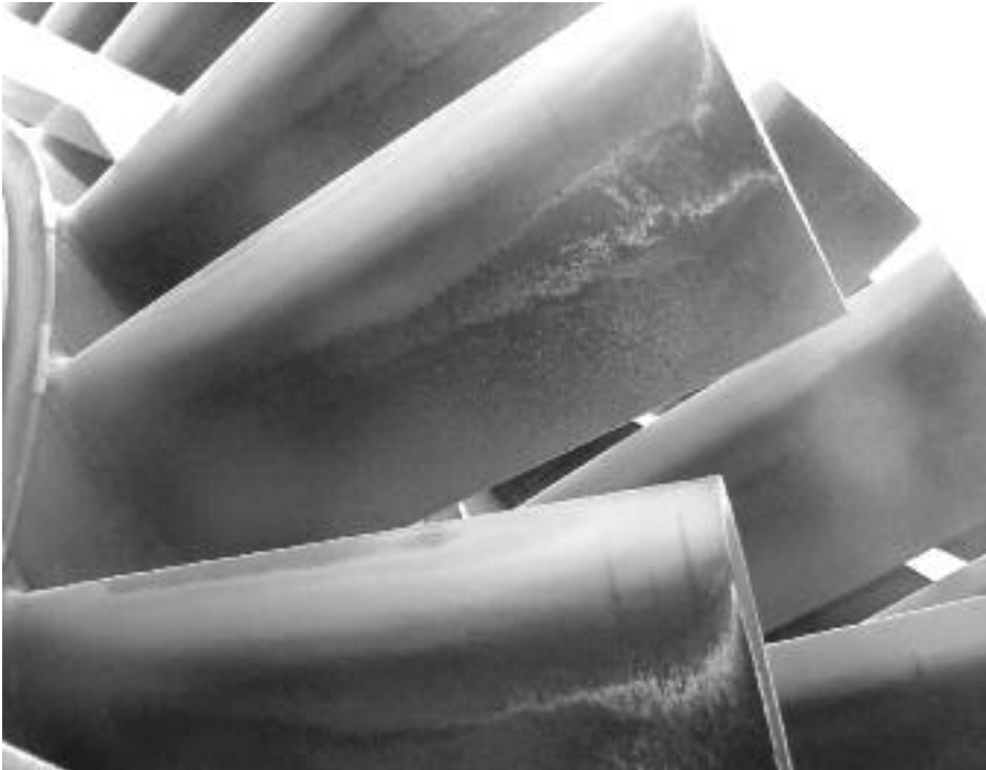
FIGURE 9.3. Deposits on the suction side of a compressor rotor. Deposits are visible in an area (halfway between leading and trailing edges) where the flow across the blade's suction side probably transitions from laminar to turbulent flow.
