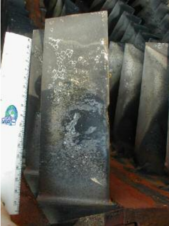
FIGURE 6.8. Degraded compressor blade.
