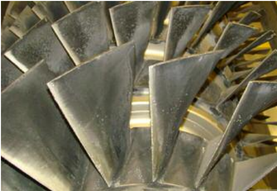
FIGURE 9.2. Salt deposits on compressor blades after 18,000 hours of operation. This is the view on the suction side. There are fewer deposits near the leading edge and in the hub region.
