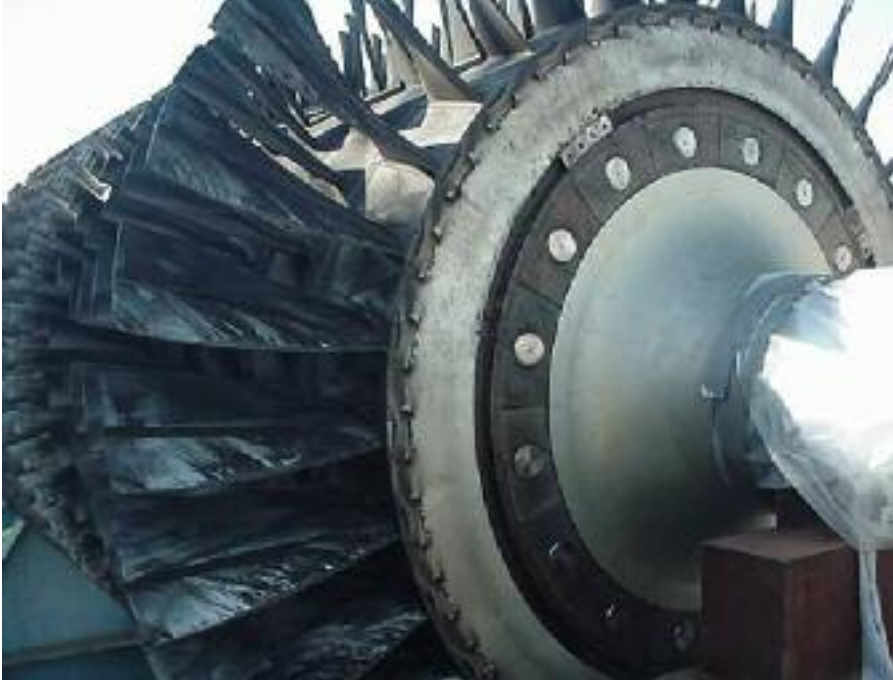
FIGURE 9.6. Oily deposits on axial compressor blades from bearing oil leakage on a large heavy duty gas turbine (Meher-Homji et al. , 2009). Oil streaks originate at the hub region and are distributed over the airfoil by centrifugal forces and blade boundary layer shear stresses.
