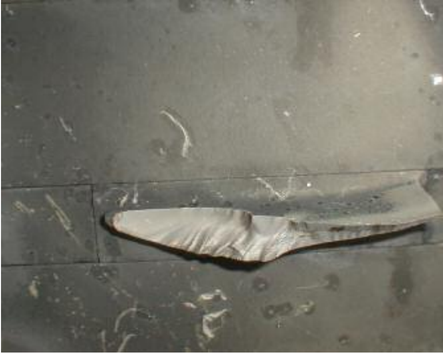
FIGURE 6.2. Compressor blade failed due to flutter-induced high-cycle fatigue.
