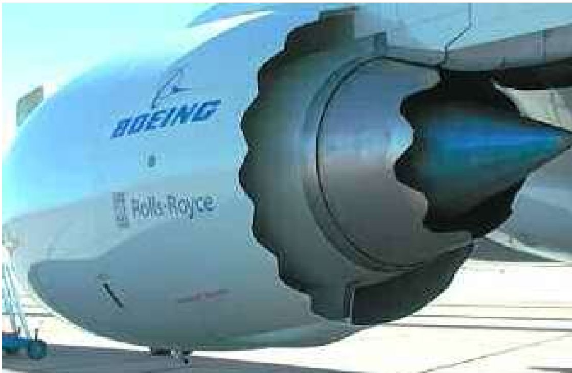
FIGURE 1.2. A Rolls-Royce Trent 800 gas turbine with serrated nozzle to reduce engine noise. The serrated nozzle reduces gas turbine noise on take-off and landing by 20 per cent (Bryanston-Cross, 2010).
