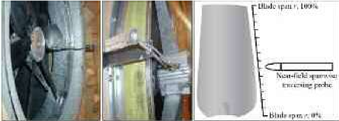
FIGURE 4.4. Microphone arrangement for inlet near-field measurements (left) and outlet near-field measurements (middle) of fan noise (Bianchi et al. , 2009a). The microphone used for outlet near-field measurements could be traversed from the blade hub to tip, right.
