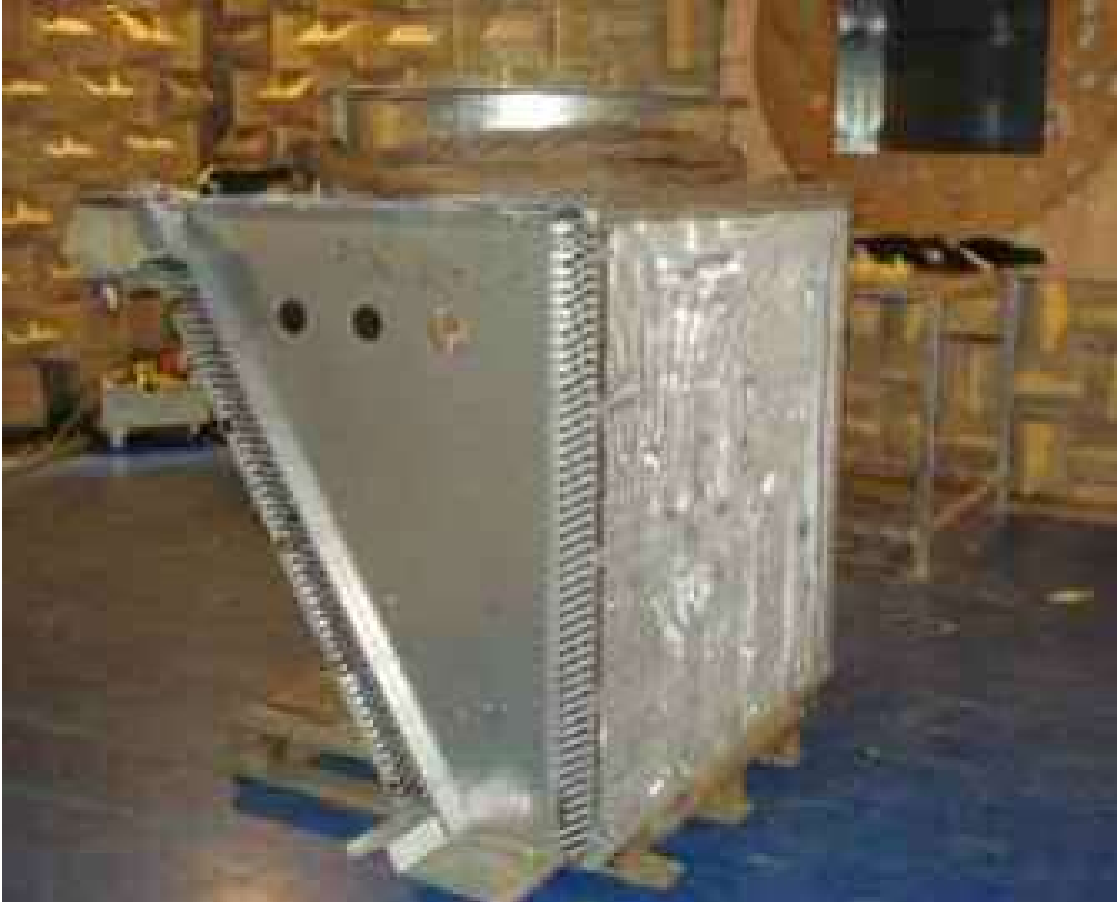
FIGURE 13.4. The studied fan installed over a compact cooling unit's tube bank that is located in a semi-anechoic chamber to facilitate fan performance and noise measurement. When installed over the compact cooling unit's tube bank, the fan inlet flow draws through the unit, passing over a tube bank.
