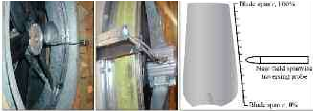
FIGURE 2.4. Microphone arrangement for the fan noise's inlet near-field measurements (left) and outlet near-field measurements (middle). The microphone that the authors used for outlet near-field measurements could be traversed from the blade hub to tip (right).
