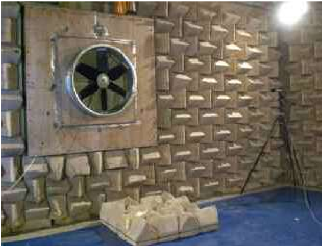
FIGURE 12.2. The standardised airway test rig set-up in a semi-anechoic chamber with a Type A (fan downstream from a plenum chamber with a free outlet) fan installation.
