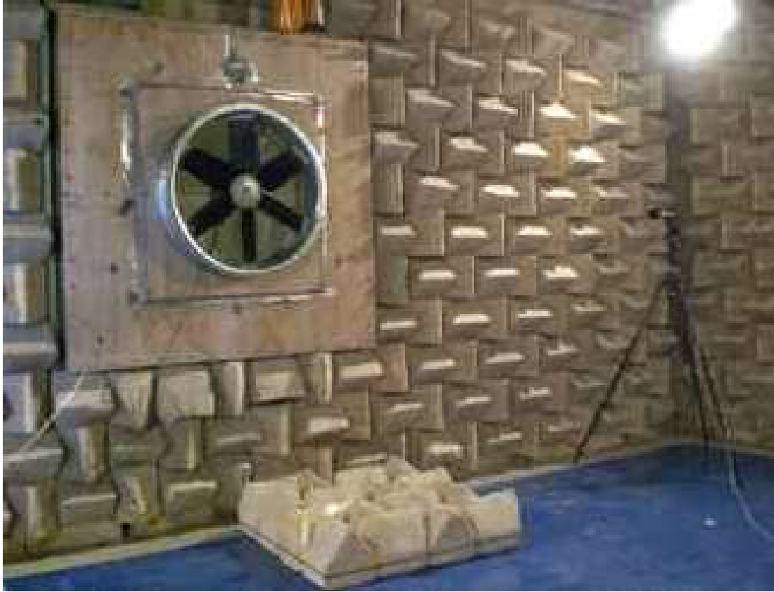
FIGURE 13.3. The standardised airway test rig set-up in a semi-anechoic chamber with a Type A (fan downstream from a plenum chamber with a free outlet) fan installation.
