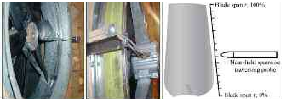
FIGURE 3.4. Microphone arrangement for inlet near-field measurements (left) and outlet near-field measurements (middle) of fan noise (Bianchi et al. , 2009). The microphone used for outlet near-field measurements could be traversed from the blade hub to tip, right.
