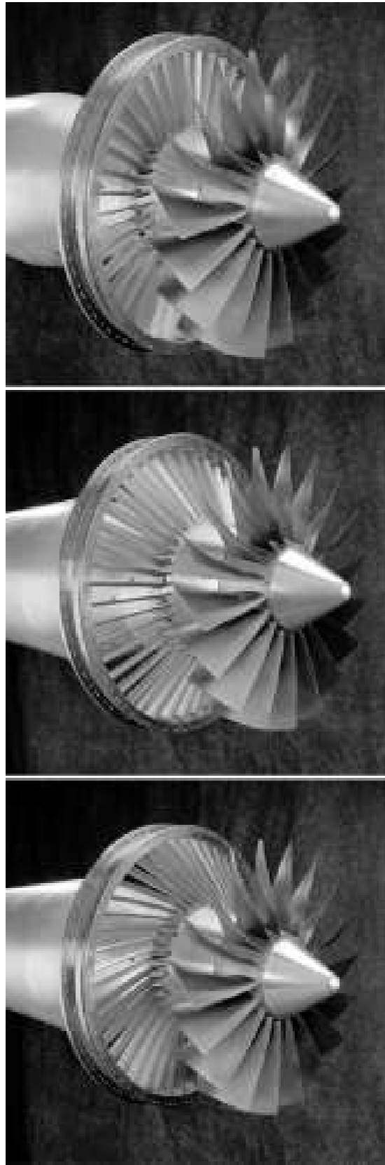
FIGURE 1.1. A base-line fan (top), with vane sweep (middle) and vane sweep and lean (bottom) (Woodward et al. , 2001). Swept vanes reduced the blade passing frequency tone amplitude and broadband noise. Stator lean reduced rotor-stator interaction resulting in a further reduction in fan broadband noise.
