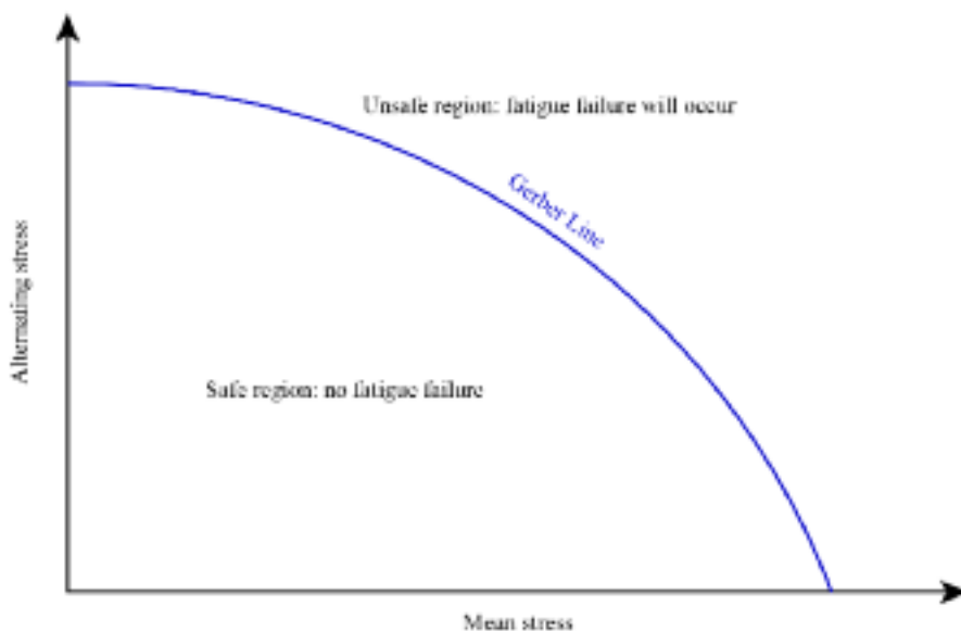
FIGURE 2.7. The curve of best fit through the limiting combination of alternating and mean stress is the Gerber Line (Gerber, 1874). Any combination of mean and alternating stress that falls outside the Gerber Line will result in a fatigue failure.
