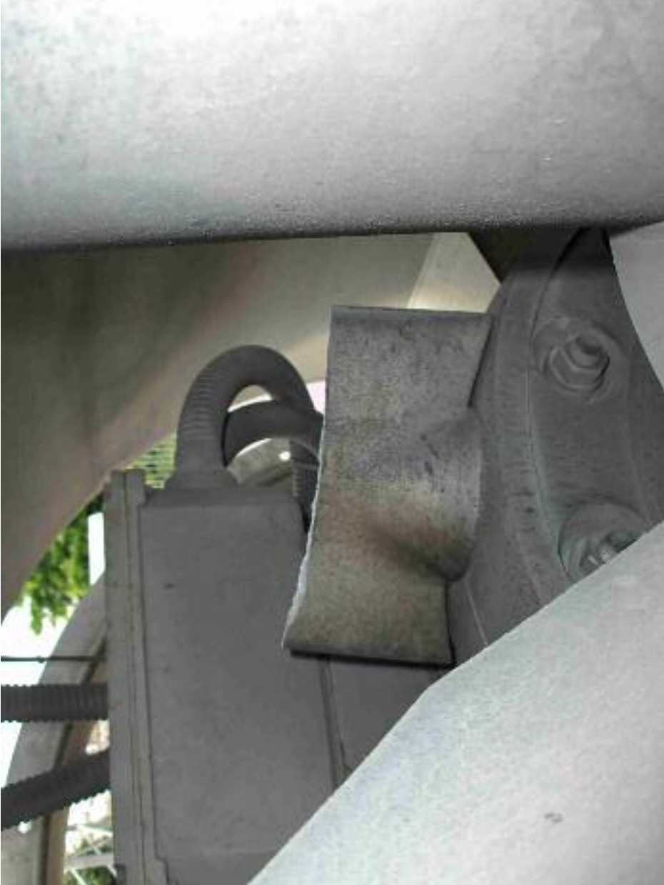
FIGURE 1.3. An example of a fan blade with a blade mechanical failure at the root aerofoil interface. This fan operated for approximately ten hours in rotating stall before the mechanical failure (Sheard and Corsini, 2011).
