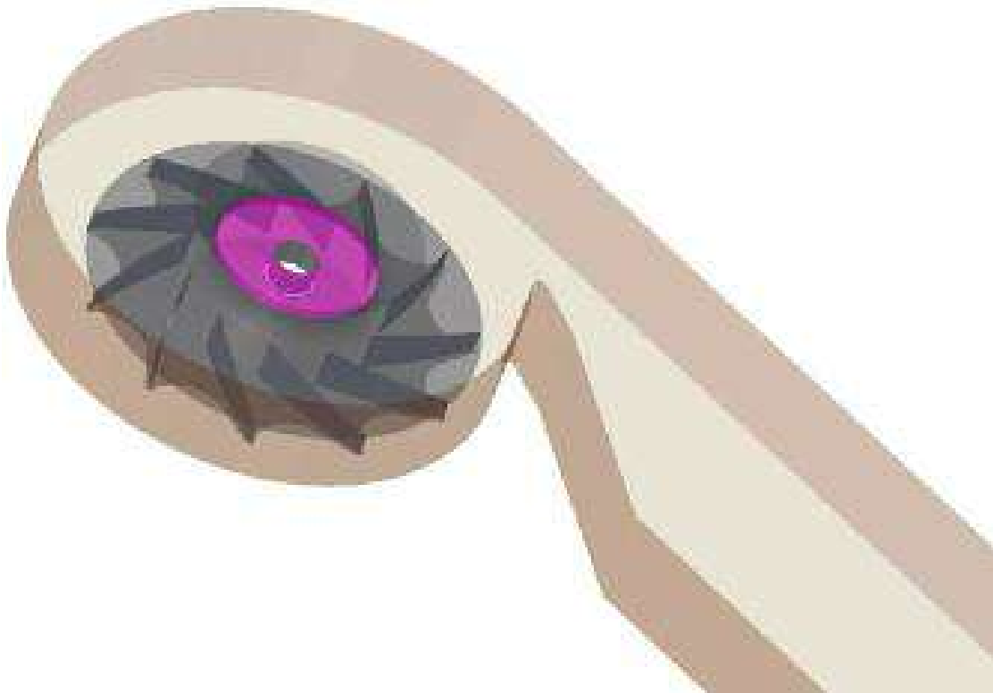
FIGURE 11.2. The modelling technique adopted modelled one half of the double inlet – double width impeller. The computational domain was split into three parts: an inlet region (shown in purple), an impeller region (shown in black) and a volute casing region (shown in grey).
