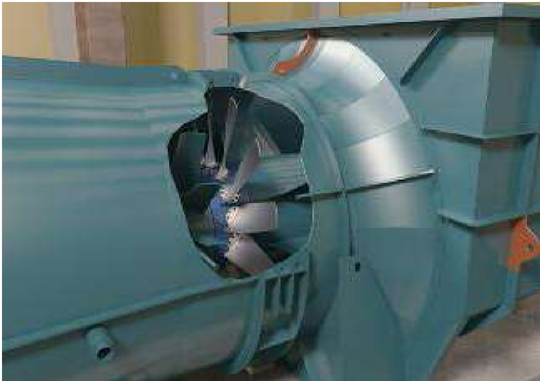
FIGURE 9.1. A cut-away view of the studied fan illustrating the variable pitch in motion blades, their inlet and outlet guide vanes. This family of fans is configured with an inlet box that turns the flow through 90 degrees. The flow into the inlet box is vertically down and the flow out is horizontal.
