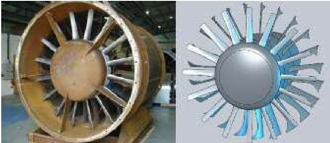
FIGURE 4.1. A prototype 2.24 metre diameter unidirectional 1,500 rpm fan named JFM 224, left and the computer aided design model that we used to define fan geometry, right. We developed the fan JFM 224 for application in railway tunnel and metropolitan metro ventilation systems. We designed this prototype for dual use: ventilating the tunnel system during routine operation and clearing 400°C gas and smoke for two hours in the event of a tunnel fire (Sheard et al. , 2009).
