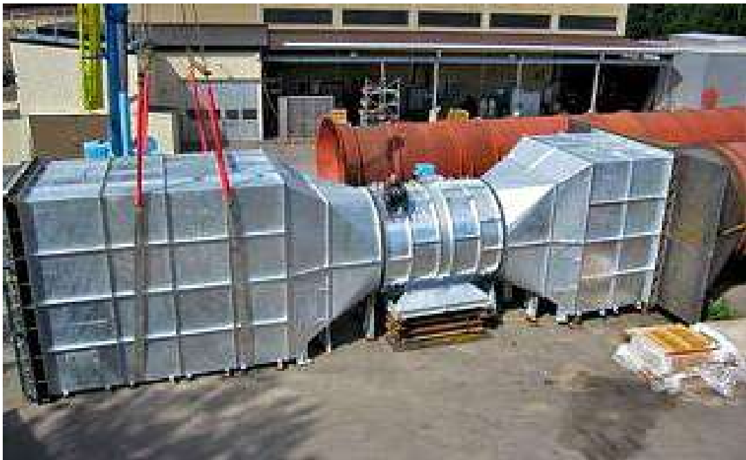
FIGURE 8.11. The first production Marmaray 2.8 metre two-stage double-ended motor fan, transform, silencer and damper package set up prior to its aerodynamic and acoustic test.
