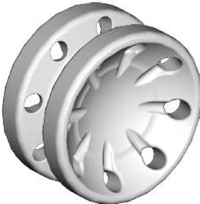
FIGURE 7.16. Sheard and Rhoden's (2012) bearing separator concept.
