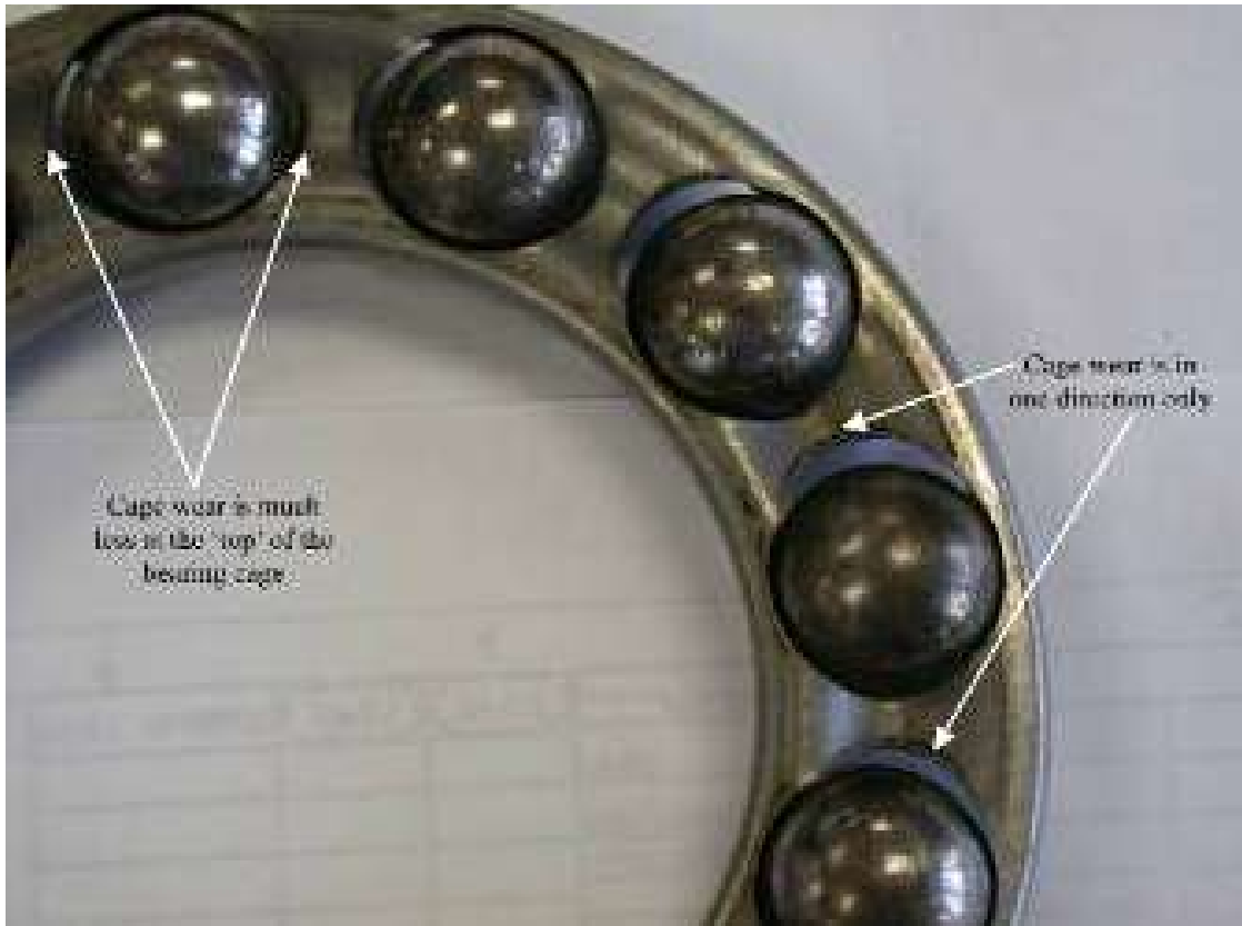
FIGURE 7.15. Wear in a traditional 'cage' bearing separator that occurs as a consequence of mechanical loads on blade bearing balls. Pitch-wise total pressure variations induce the mechanical loads.
