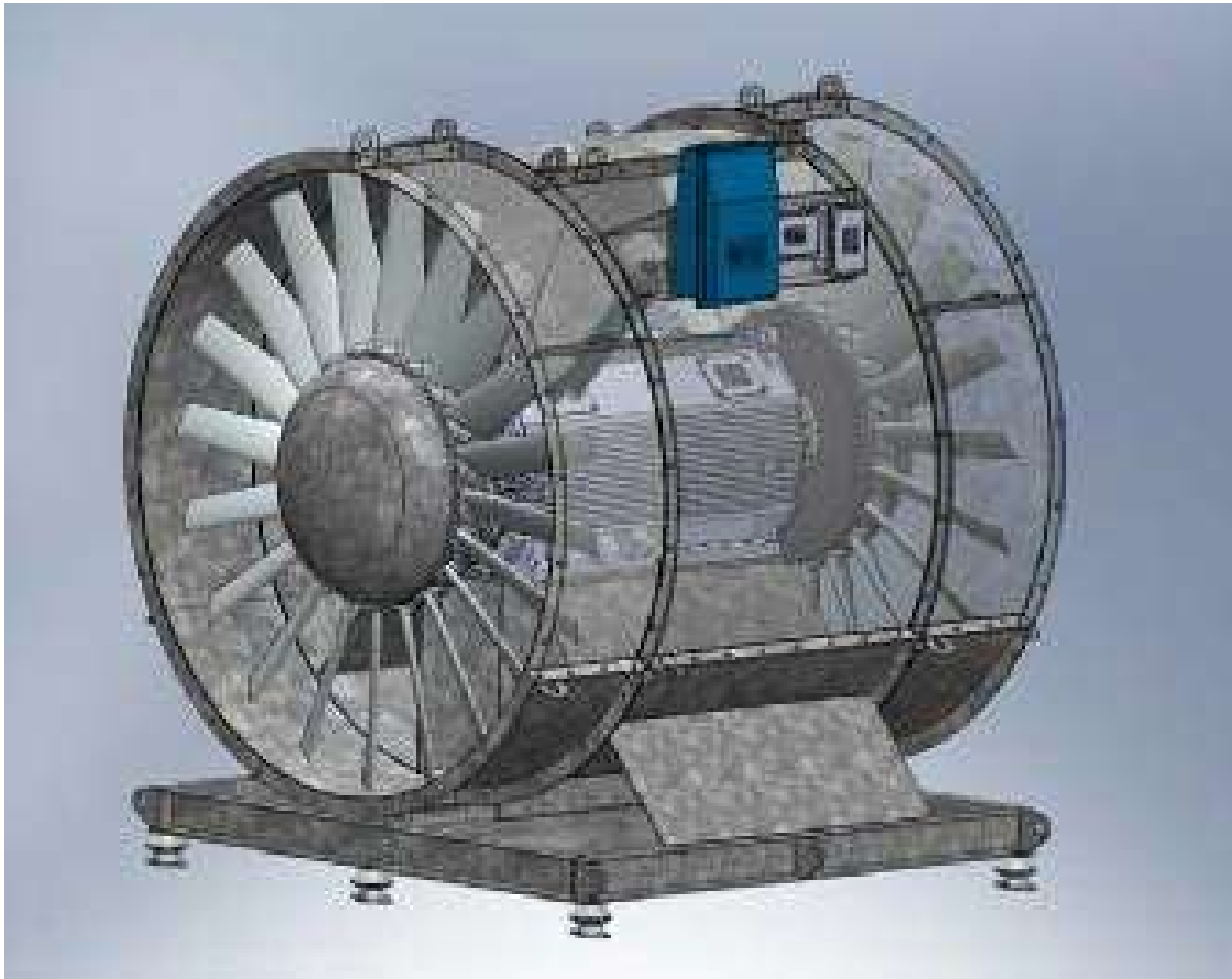
FIGURE 8.7. A computer aided design model of the horizontal 2.8 metre two-stage double-ended motor fan designed for the Marmaray project.
