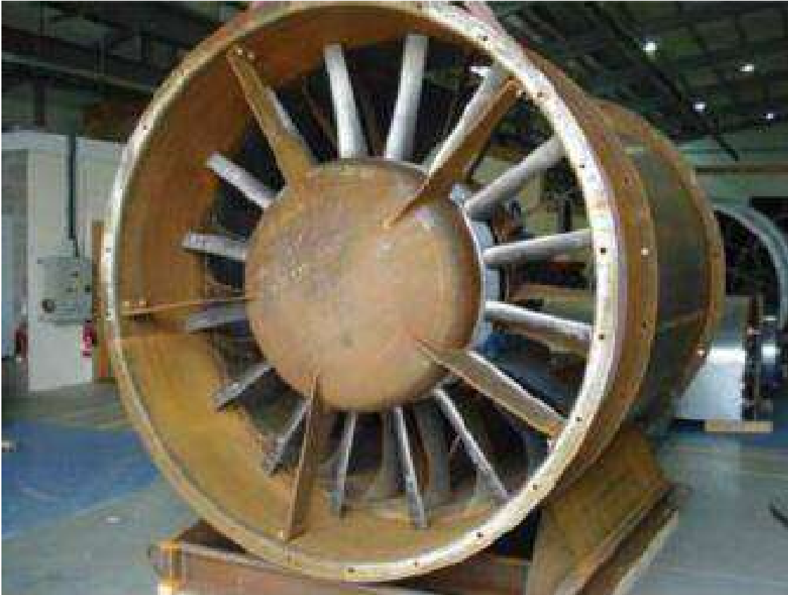
FIGURE 3.8. A prototype 2.24 metre diameter unidirectional 1,500 rpm fan named JFM 224 and intended for application in railway tunnel and metropolitan metro ventilation systems. This prototype was designed for dual use, ventilating the tunnel system during routine operation and clearing 400°C gas and smoke for two hours in the event of a tunnel fire (Sheard et al. , 2009).
