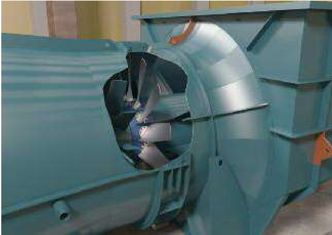
FIGURE 10.1. A cut-away view of the studied fan illustrating the variable pitch in motion blades, their inlet and outlet guide vanes. This family of fans is configured with an inlet box that turns the flow through 90 degrees. The flow into the inlet box is vertically down and the flow out is horizontal.
