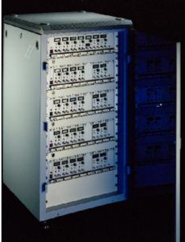
FIGURE 7.7. A 20-channel capacitive clearance measurement system ground station.
