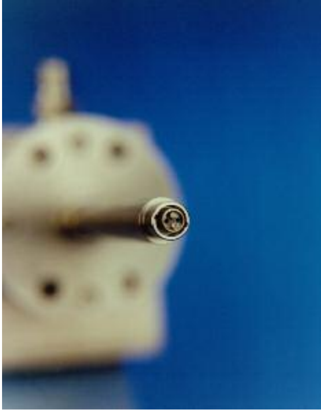
FIGURE 6.5. A close-up view of a probe tip, with electrode (bottom), capacitance probe (top) and cooling holes (left and right).
