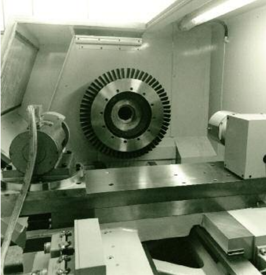
FIGURE 5.7. The computer numerically controlled lathe fitted with a grinding spindle, prototype measurement head, datum disc and Pratt & Whitney JT8 stage 11 bladed compressor disc.
