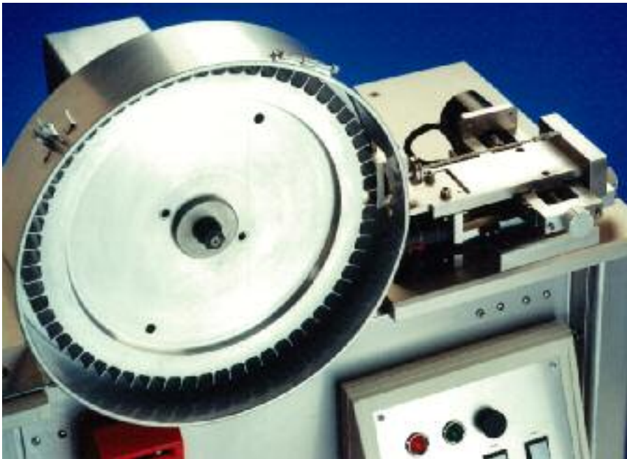
FIGURE 7.5. Capacitance probe mounted in the calibration rig. The capacitance probe is mounted on a traverse mechanism (right) with a reproduction of the gas turbine casing around the probe tip at the equivalent of 3 o'clock over the calibration disc blades.
