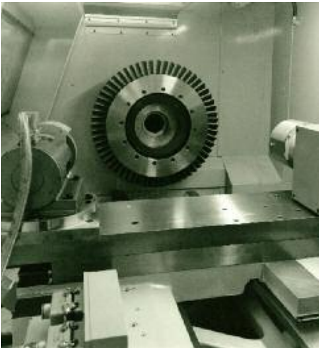
FIGURE 4.7. The prototype measurement head fitted to a computer numerically controlled (CNC) lathe with a Pratt & Whitney JT8 stage 11 compressor disc and blade set.
