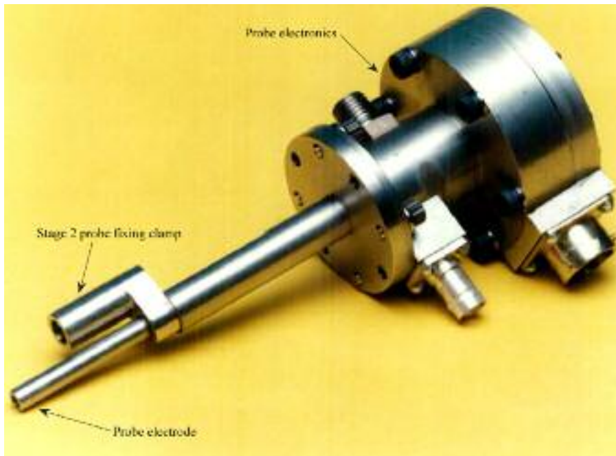
FIGURE 1.1. An example of Amsbury and Chivers' (1978) design of electromechanical clearance measurement system probe and actuator.
