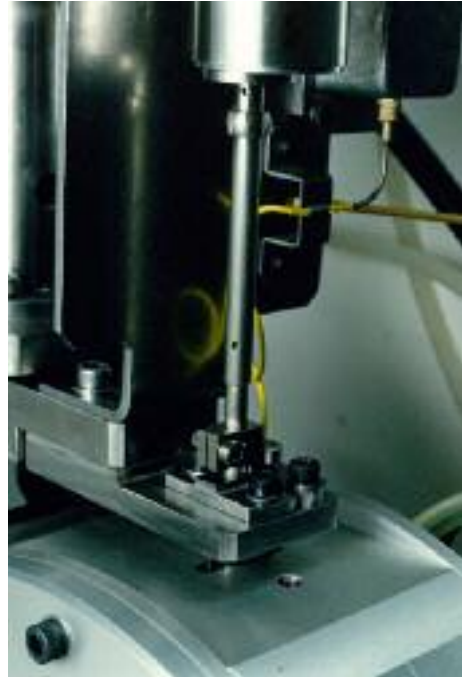
FIGURE 3.8. Close-up view of the traverse actuator mounting on the spinning rig housing showing the clamping arrangement of the capacitance probe and touch wire.
