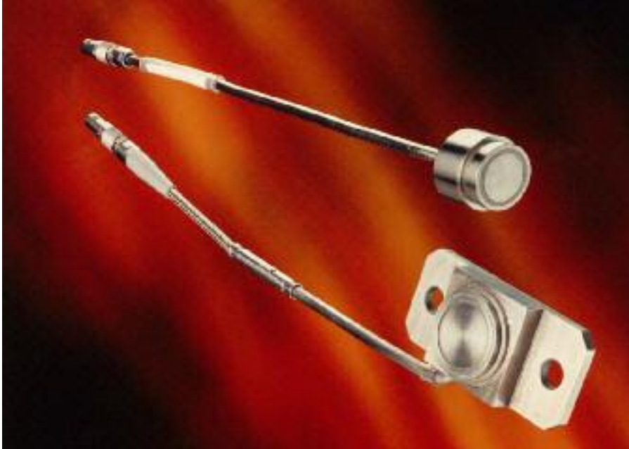
FIGURE 9.1. Traditional tri-axial capacitive sensor (top) originally developed by Chivers (1989a) and the new technology (NT) capacitive sensor (bottom) originally developed by Sheard and Lawrence (1998). This example of the new technology capacitive sensor was designed with side entry cable.
