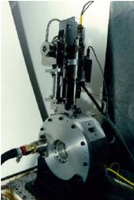
FIGURE 3.7. The spinning rig used to evaluate performance of Chivers’ (1989a) capacitive clearance measurement system.
